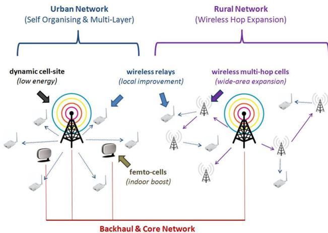
Fig. 2. Advanced 4G LTE-A Architecture for Urban and Rural environments.
