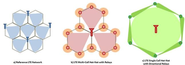
Fig. 3. Reference and Dynamic Deployments: a) Reference micro-cell deployment; b) Macro-sectorized-cell deployment with low power relays; c) Macro-single-cell deployment with high power directional relays.
